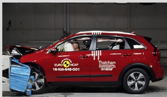
Frontal offset test at 64km/h
