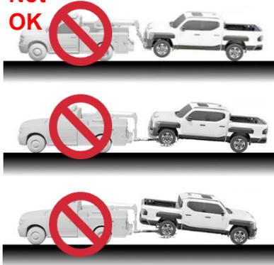
Notice : Do not tow with sling-type equipment. Do not tow the vehicle with the front wheels on the ground as this may cause damage to the vehicle
