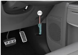
Pull the hood release lever to unlatch the hood (1).
