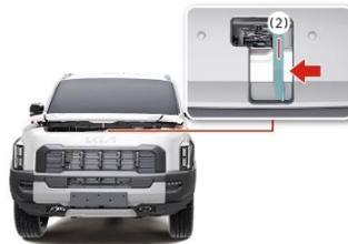
Go to the front of the vehicle, raise the hood slightly, push up the hood release lever inside of the hood center and lift the hood (2).
