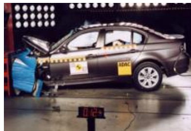
Offset crash test at 64km/hr
