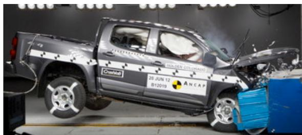
Offset crash test at 64km/h (Colorado Utility)
