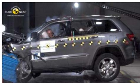
Offset crash test at 64km/h
