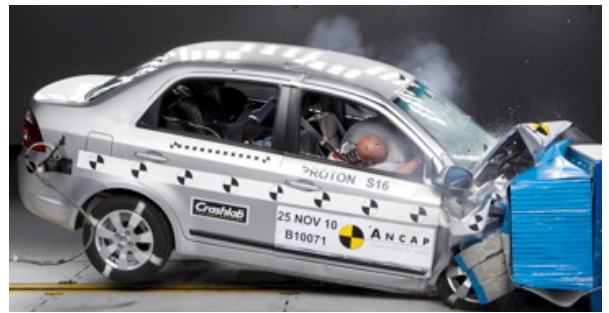
Offset crash test at 64km/h
