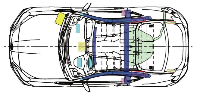
Note: The Rescue Sheet depicts a LHD vehicle (as allowed under the ISO 17840-1). All components (other than steering wheel and passenger airbag) are located in the same position in the Aust/NZ RHD model.
