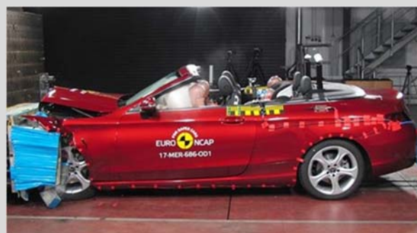
Frontal offset test at 64km/h
