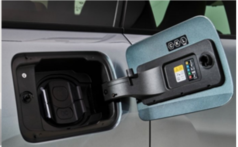
High-voltage charging socket on the rear right side panel
