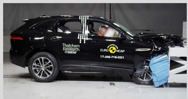
Frontal offset test at 64km/h
