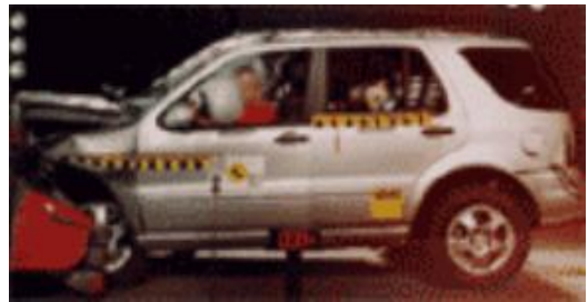
Offset crash test at 64km/hr
