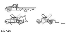
Do not tow a vehicle that has been involved in an accident on its drive axles.
