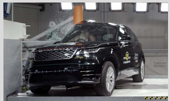
Oblique pole test at 32km/h
