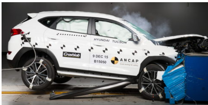
Frontal offset test at 64km/h
