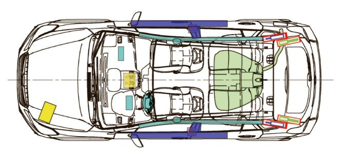
Note: The Rescue Sheet depicts a LHD vehicle (as allowed under the ISO 17840-1). All components (other than steering wheel and passenger airbag) are located in the same position in the Aust/NZ RHD model.
