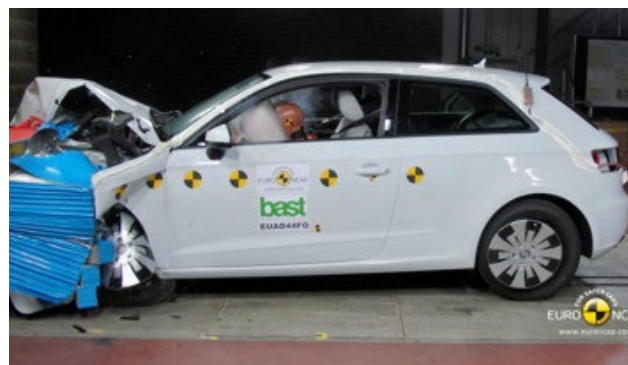
Frontal offset test at 64 km/h (Euro NCAP)
