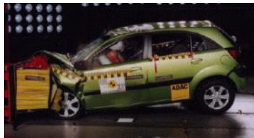
Offset crash test at 64km/hr
