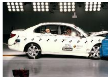
Offset crash test at 64km/hr
