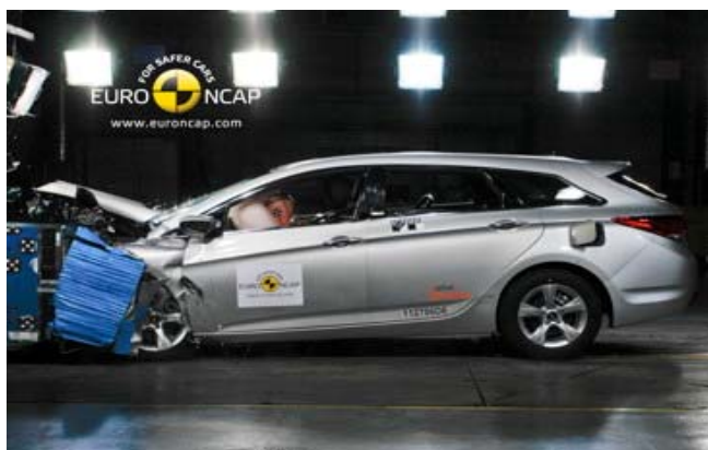
Frontal offset test at 64km/h
