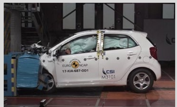
Frontal offset test at 64km/h
