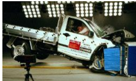
Offset crash test at 64km/hr
