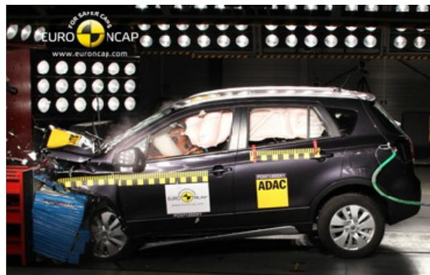
Frontal offset test at 64 km/h (Euro NCAP)
