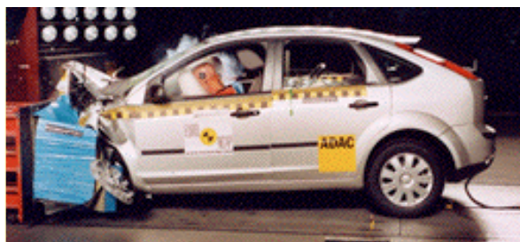
Offset crash test at 64km/h
