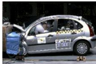
Offset crash test at 64km/hr
