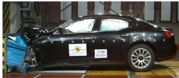
Frontal offset test at 64 km/h (Euro NCAP)
