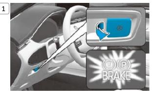
1. Chock the wheels and pull the switch to set the parking brake.
