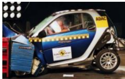
Offset crash test at 64km/hr
