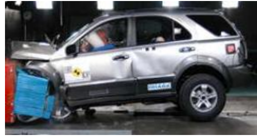
Offset crash test at 64km/hr
