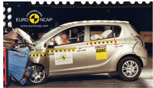
Offset crash test at 64km/h
