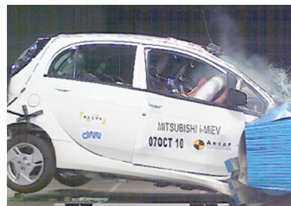
Offset crash test at 64km/h
