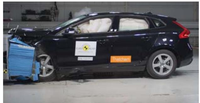
Frontal offset test at 64 km/h (Source: Euro NCAP)
