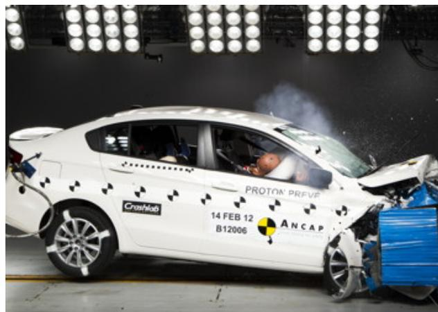
Frontal offset test at 64 km/h
