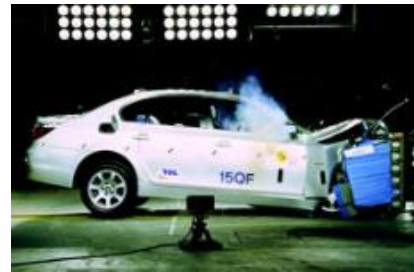
Offset crash test at 64km/hr
