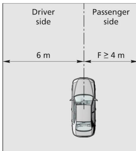
The free space  $F$  between the VUT path and the mounting facility shall be  **$F \geq 4\text{m}$** .
