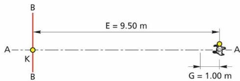
**Figure 7-7 CPTAfo scenario – VUT right turn, pedestrian crossing from farside**
