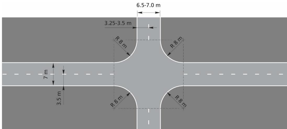
**Figure 6-1: Layout of junction and the connecting lanes**
