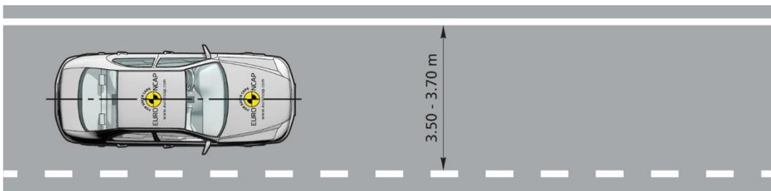
**Figure 6-2: Layout of the lane markings**
