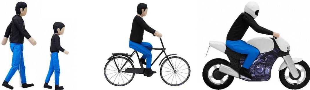
**Figure 5-1: Euro NCAP VRU Targets (EPTa, EPTc, EBTa and EMT)**
