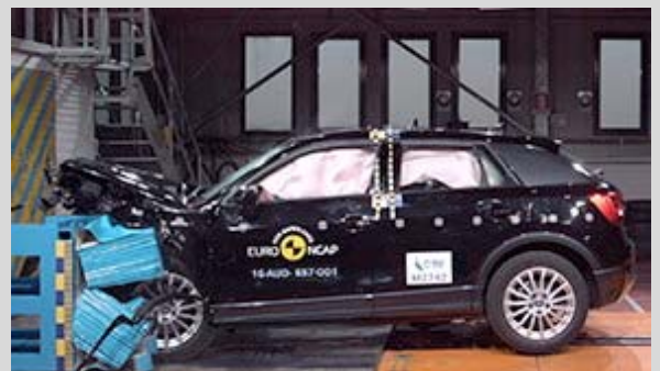
Frontal offset test at 64km/h
