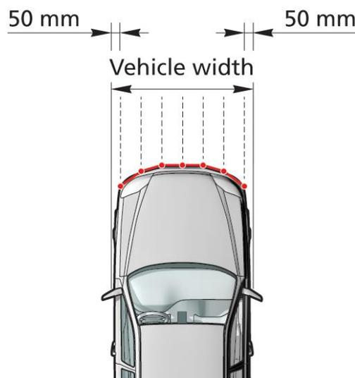
Figure 3-4 VUT Front bumper profile
