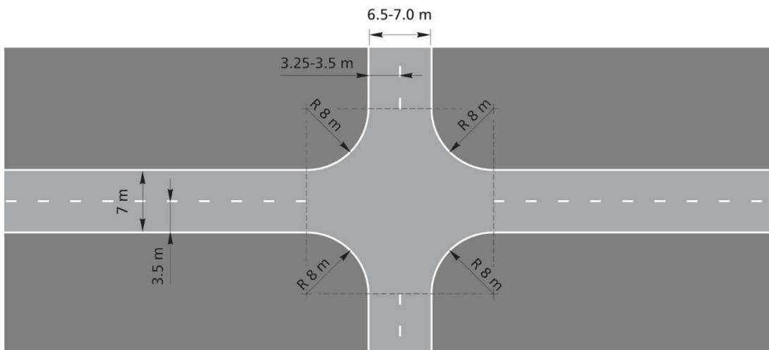
Figure 7-1: Layout of junction and the connecting lanes
