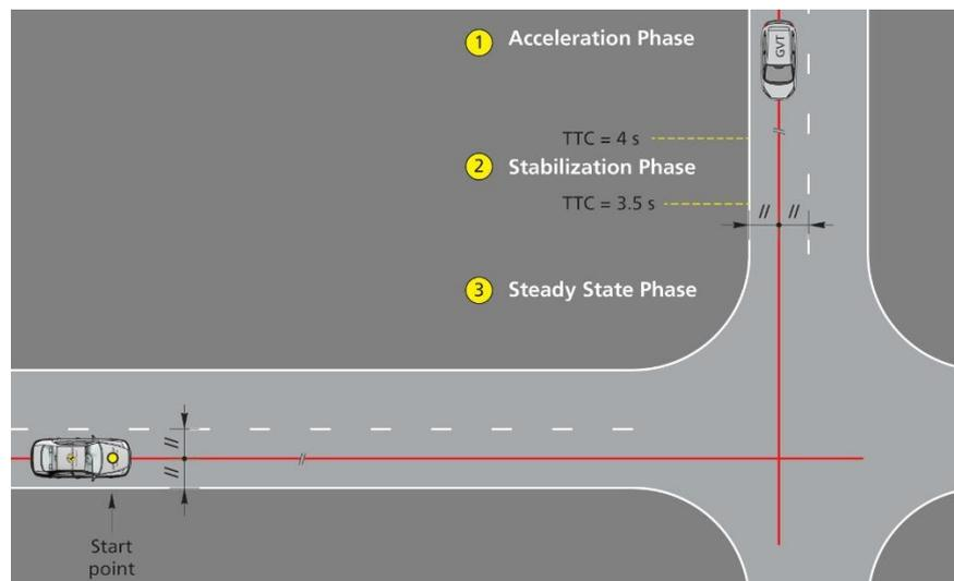
Figure 8-7 Straight Crossing Path VUT and GVT paths
