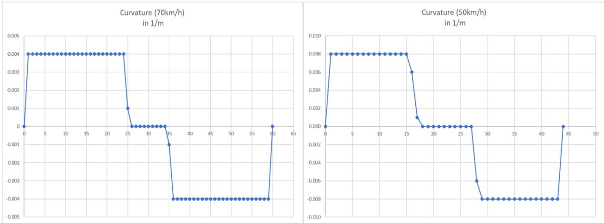
Figure 8-13 CCFhol curvature values at 70 and 50 km/h
