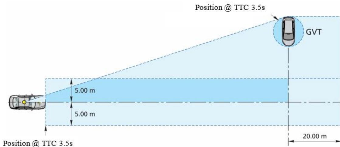
**Figure 7-3: Free space requirements – CCC Farside Test**
