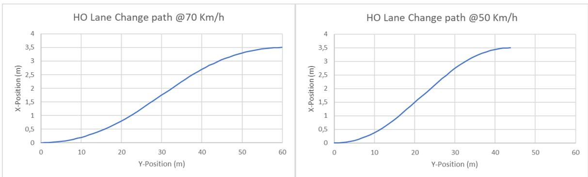
Figure 8-12 CCFhol path at 70 and 50 km/h
