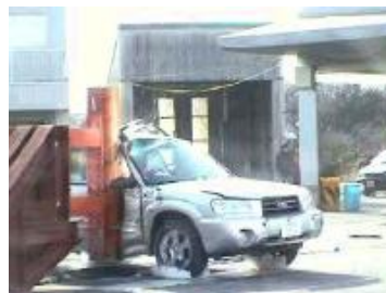
Offset crash test at 64km/hr
