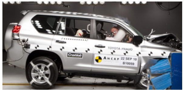
Offset crash test at 64km/h
