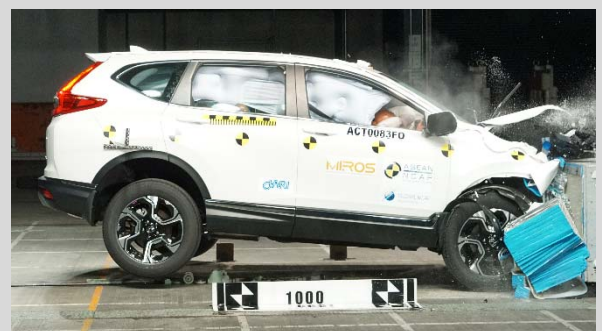
Frontal offset test at 64km/h
