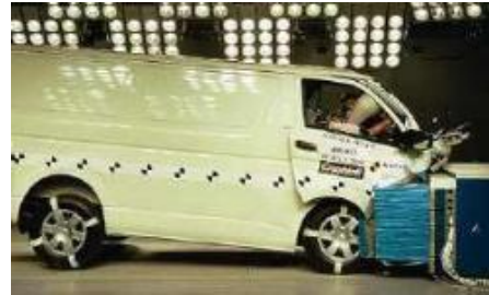
Offset crash test at 64km/hr
