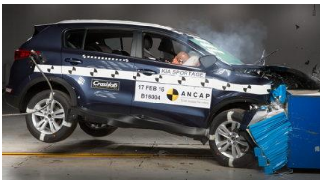
Frontal offset test at 64km/h
