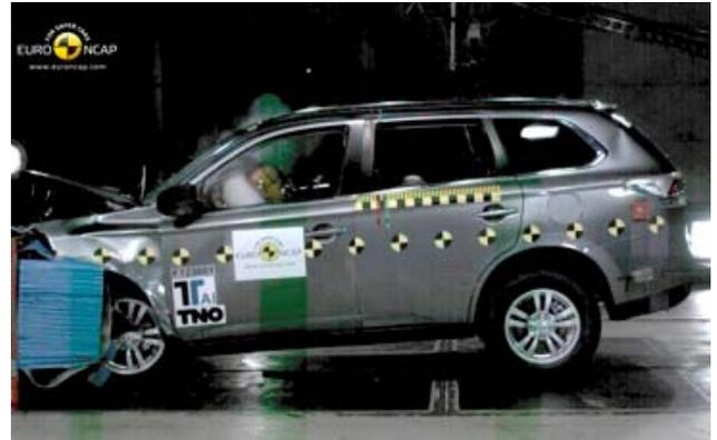
Frontal offset test at 64 km/h (Euro NCAP)
