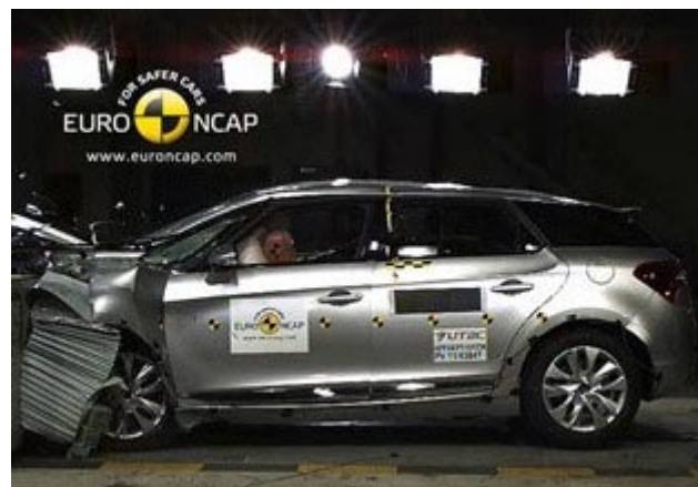
Frontal offset test at 64 km/h
