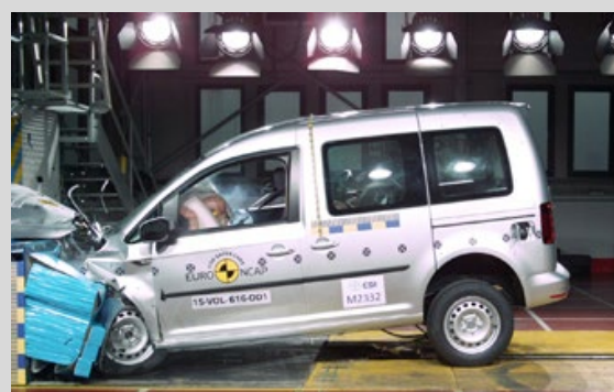
Frontal offset test at 64km/h
