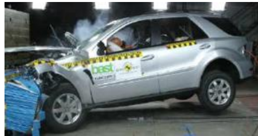
Offset crash test at 64km/hr
