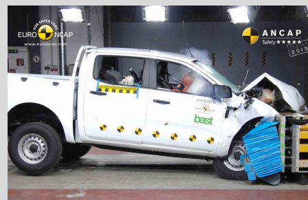
Frontal offset test at 64km/h
