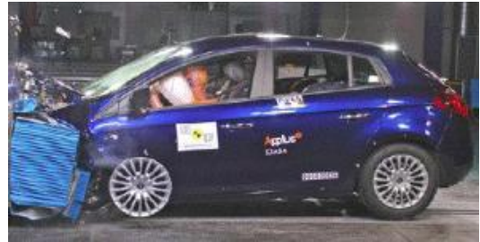
Offset crash test at 64km/hr
