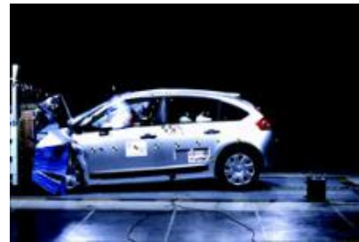
Offset crash test at 64km/hr
