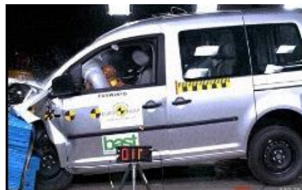
Offset crash test at 64km/hr
