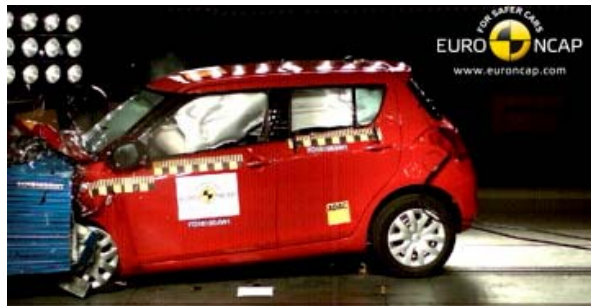
Offset crash test at 64km/h
